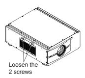
Remove the dirty filter; you can clean it directly using water. Leave it to dry before replacing it for further use. If the filter is broken, purchase a new one to replace it.
